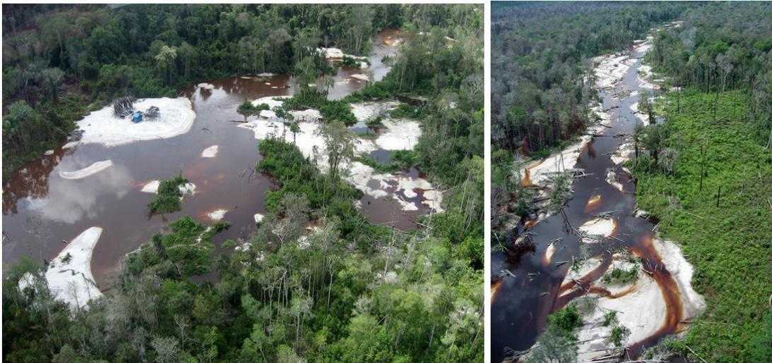
**Figure 4-6 One of a Myriad of workings along small river courses in Kalimantan. Hundreds of kilometres of small drainages have been worked for gold and zircon like this. It is more difficult to detect than large workings such as those shown in Figure 4-2 due to confusion with natural river courses. Note also the colour of the water demonstrating its very high dissolved organic carbon content – known to be a strong complexing agent of Mercury.**
