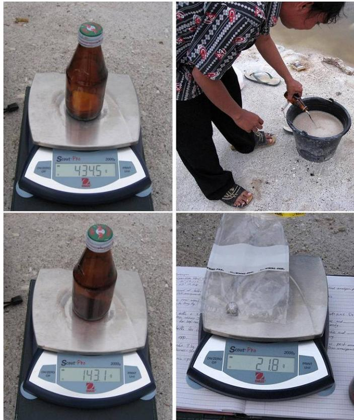
**Figure 4-8** directly weighing and calculating amounts of mercury consumed during the amalgamation process and gold refining. This method revealed that on average for the region 1.5 units of mercury are consumed per unit of gold recovered and that 30% of the mercury is lost to the tailings and the rest lost to the atmosphere when heated later in the gold shops to produce the gold.
