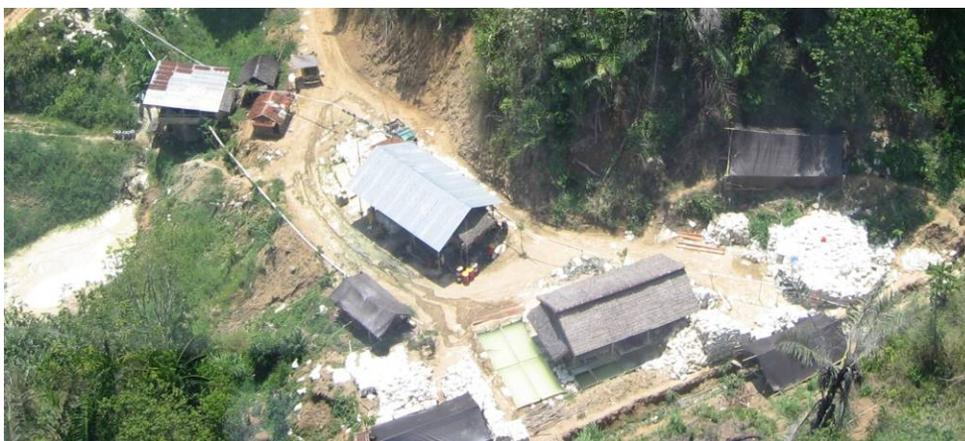
**Figure 4-2b Aerial Photography taken by Kevin Telmer in 2006 shows ASM methods and their impacts in Indonesia. (iii) the vastly altered landscape resulting from 15 years of sluicing operations in Galangan (above); (iv) cyanide processing tanks (roofed), bags of ore, and cyanide and mercury rich tailings, near Kotamobagu, Sulawesi (below).**
